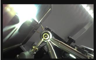
State of the art Bruker D8-Venture X-ray Machine equipped with a CMOS  $(10 \times 10 \text{ cm}^2) \text{ detector.}$
